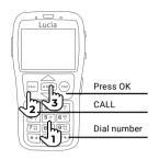
Press the repeat speech button on the right edge of the phone at any time to hear the numbers you have typed. The number you are dialling will also be repeated once you press the CALL button.
